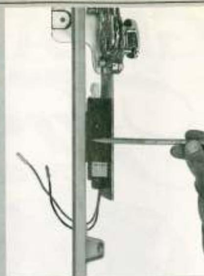
**6** When determining where to drill the holes to mount the actuator, you must consider the clearances needed to avoid obstruction of the window felt-channel that mounts inside the door and the travel length of the actuator's plunger. Here is the completed latch assembly with the felt channel mocked up to show perspective.
