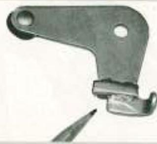
**10** Two other specialty brackets must be welded to the opening lever. The first one is a mounting sleeve that will secure the steel cable to the lever. The second one is a bracket that will disengage the locking lever when opening the door from the inside.
