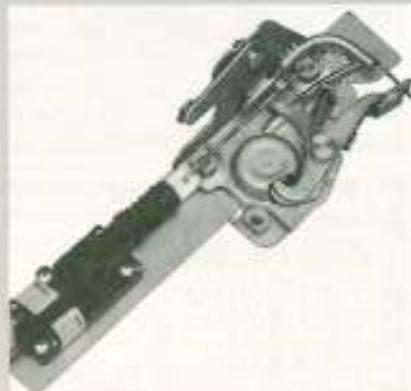
**14** Now that the latch assembly has been modified to accept an actuator, the actuator can be permanently installed. The hook on the connecting rod is hooked to the actuator's plunger, and the other end of the connecting rod is slid through the hole in the pin on the locking latch. Then three low-profile bolts are installed to secure the actuator to the mounting plate as shown.
