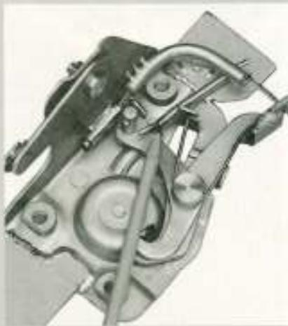
**13** Due to the pull of gravity and friction between the opening latch and the locking latch, a small spring will need to be affixed to the locking latch to keep the latch from unlocking on its own. This means that the locking latch will always remain in the locked position. Here, we show the spring in place and connected to the locking latch.
