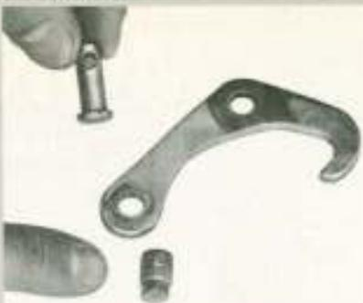
**12** On the locking latch, the old engagement pin is ground out with a die grinder, and a new longer pin is welded into the same place. This pin is going to be used to affix the connecting rod from the actuator. A hole is drilled in the center of the pin at a height where the connecting rod is geometrically operational with the actuator.
