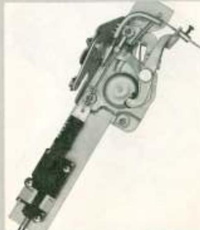
**17** Here is what the final latch assembly should look like after the latch has been converted to power door locks. Note how the locking and the opening mechanisms are independent of each other now.
