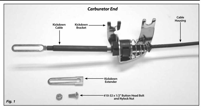
Step 11: To adjust the cable, release the latch on the black housing by pushing it up from the bottom. Fig. 5 If you cannot get it to release by hand, you may be able to pry the latch up with a screwdriver. Move the throttle to the wide open position and hold it there. Push the latch back down to lock the cable housing into position. Release the throttle.
