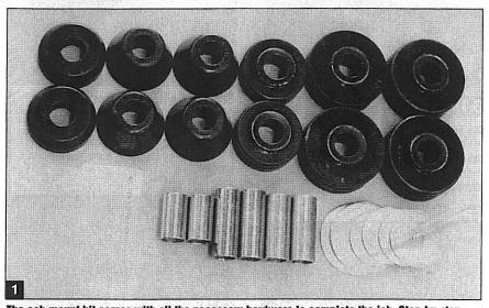
The cab mount kit comes with all the necessary hardware to complete the job. Step-by-step instructions are also included to point out where the different bushings go.
