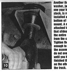
**Another thick** washer, just like the one your truck had stock, is reinstalled at the bottom of the lower mount. A nut is then attached to the bolt that slides through the entire assembly from the cab floor. **Tighten the nut** enough to secure the assembly, but do not overtighten until you have finished the process on the other side of
