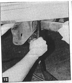
The same procedure used for removing the cab mounts applies to the core support mounts as well.
