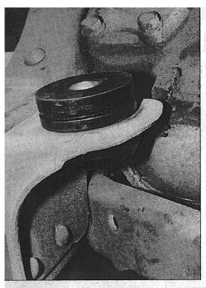
With the core support remove (done for photo purposes only), you can clearly see what the ne mounts look lik when they are properly install Now, simply reinstall the mounting bolt a you're all done and riding dow the road in greater comfor
