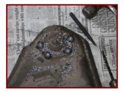
3. Step up to the 3/8" bit and drill out the heads of the rivets. Again, use cutting oil while drilling.
