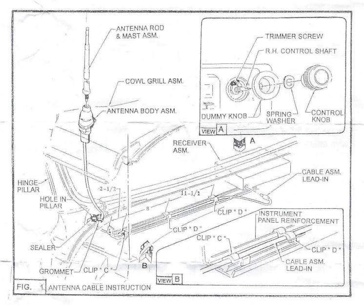
STEP 1 ROUTE CABLE ASM, LEAD-IN THRU GROMMET.
