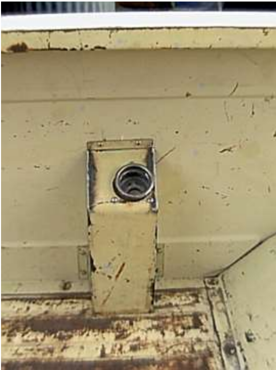
The 87 Suburban filler tube above was fitted into the modified the original gas filler cover and was located on the rear drivers rear inner bedside to smooth and clean up the outer body
