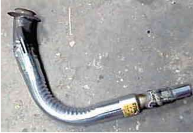
The 87 Suburban filler tube above was fitted into the modified the original gas filler cover and was located on the rear drivers rear inner bedside to smooth and clean up the outer body
