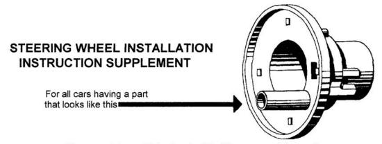
After removal of your old steering wheel, it will be necessary to remove the horn contact plunger and its spring from the plastic horn contact assembly, which should still be on your steering shaft. This horn contact plunger and spring will be replaced in the following manner:
