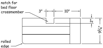
Aluminum fuel tank for 72 SWB fleet w/ steel floor material - 1/8" aluminum
