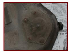
Using a 1/4" bit, drill through each of the heads and slightly into the shafts of the rivets. Use cutting oil to assist in the drilling.
