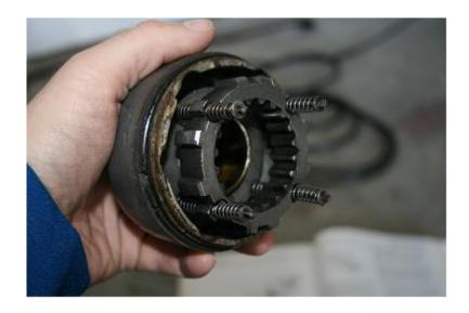
4. Remove the snap ring with a pick and a screwdriver
