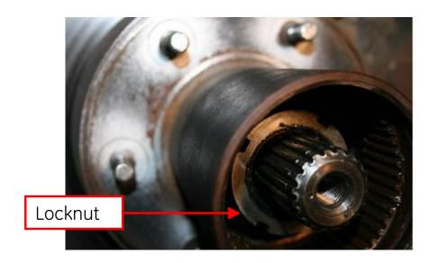
10. Remove the washer and the wheel bearing adjustment nut, the adjustment nut looks exactly like the locknut from step 8.
