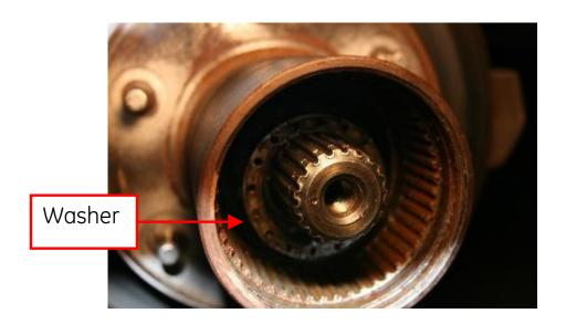
11. Remove the outer wheel bearing, there's no seal here.
