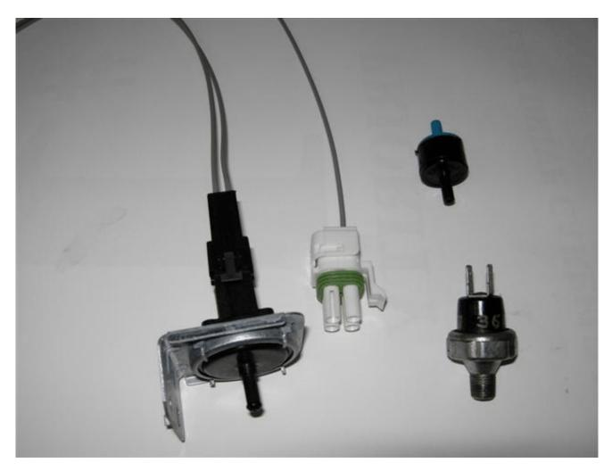
The round piece with the blue end is a vacuum restrictor. Sometimes this is needed to regulate vacuum if erratic tcc engagement occurs. This goes into the vacuum hose attaching to the vacuum switch. Blue end toward vacuum source.
