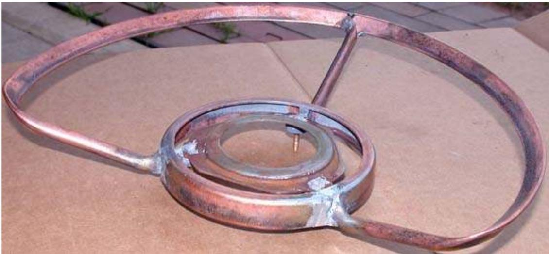
Picture 5. ZB Horn Ring. Shown on right is repair of major break in the support ring
