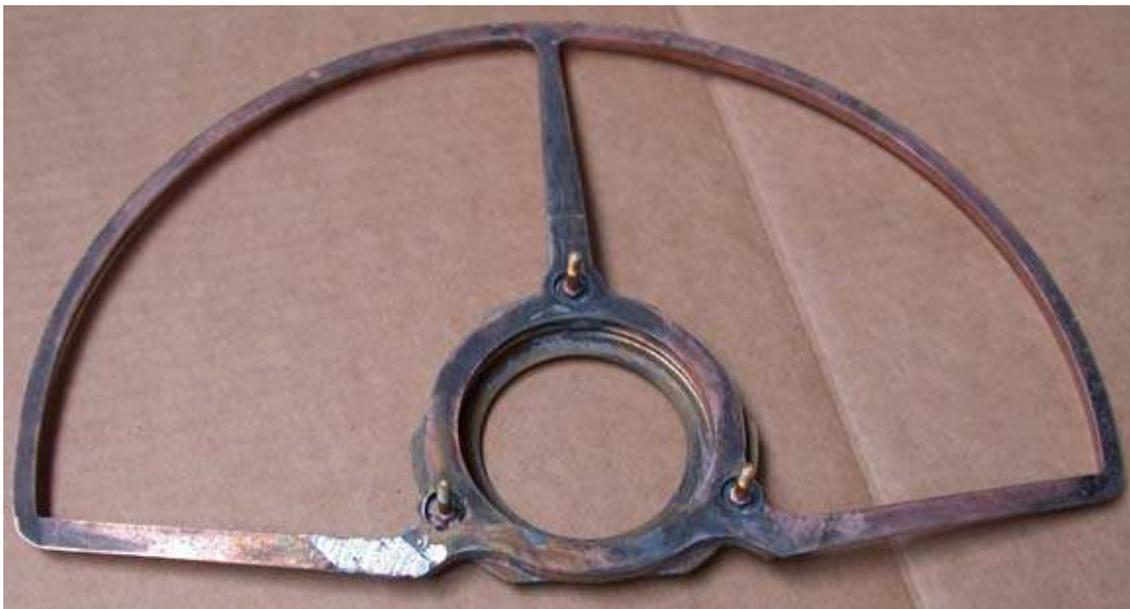
Picture 4. Underside repair. Note the three studs, they are riveted from front.
