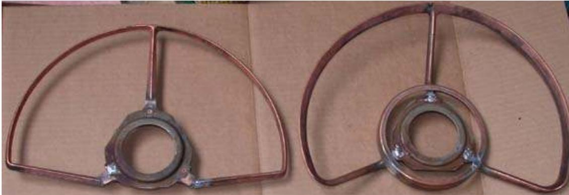
Picture 7. ZA and ZB Horn rings after initial welding of die cast and soldering of rivets
