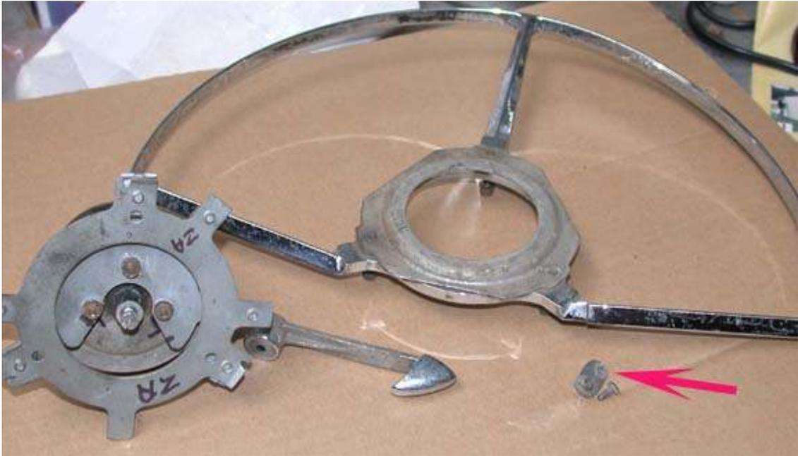
Picture 2. ZA horn ring with attachments taken off [bridging/repair plate removed]
