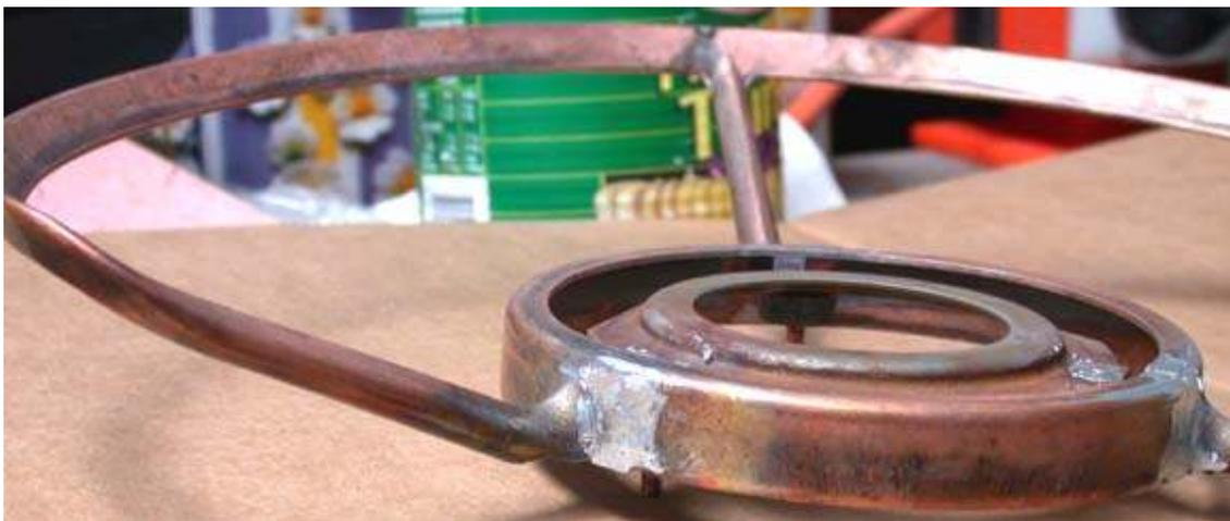
Picture 6. ZB Horn Ring. Shown on the left is repair to the fracture in the support ring
