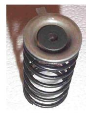
Install the screw into the spring plate and the spring over the plate. Your assembly should look like this. The flat top of the screw will bear the pressure of the spring just as the original, and the recess in the cap will prevent the screw from wandering too far from center to create problems.
