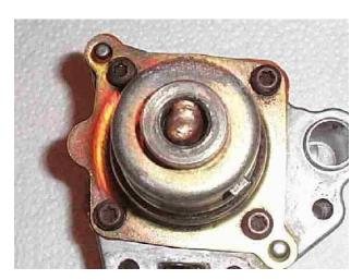
This brazed area must be drilled out to free the adjustment screw. Using the center punch, make an indentation at the center of the recess. Using this center and the inside of the recess as a bushing, drill the bronze out with a 21/64" or 'R' (0.339") drill. A 1/4" spot weld cutter also works nicely if you have access to one.
