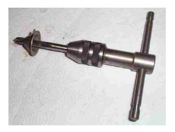
If you are using the replacement 1/4-28 screw, you must drill the hole in the spring disc with a 7/32" or #3 drill and tap 1/4-28 UNF threads for the new screw.
