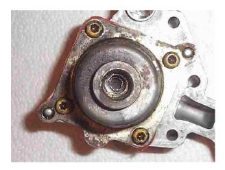
Adjust the regulator spring disc position to the same point as your original marks to begin with. Reassemble the regulator to the TBI unit in the revers order of disassembly. If there is any question about the integrity of the gaskets, replace them. Connect the fuel lines if removed and operate the fuel pump to test the system for leakage. Turning the ignition switch to the RUN position without cranking the engine should cause the fuel pump to run long enough to build pressure.
